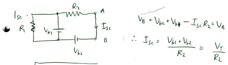
$$R_{\tau} = \frac{V_{\tau}}{I_{sc}} = R_{z}$$
