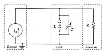
(a) Show that when  $\omega \approx 1/\sqrt{LC}$  the impedance of the parallel *LC* combination is very large, such that the signal is passed to the receiver (resistor *R*). On the hand, show that when  $\omega$  is far from  $1/\sqrt{LC}$ , the impedance of the tank circuit is very low such that signal is not passed to the receiver.
