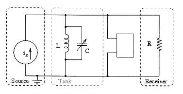
The proposed sub-circuit is shown below. Determine the equivalent resistance  $R_{eq}$  of this subcircuit. That is, find the ratio  $v/i \equiv R_{eq}$  where v is the labelled voltage across the input terminals and i is as shown in the figure. *Hint: You should find that*  $R_{eq}$  *is negative!*
